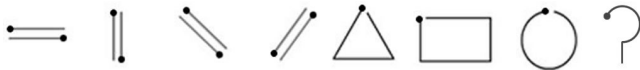
Figure 3. The eight tested unistroke gestures. The black dot indicates the start of the gesture.
