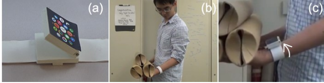
Figure 2. Watch hand unavailable: (a) Passive low fidelity prototype; (b) Watch faces the ground when the user carries an object; (c) Face orbits to the visible part of the wrist band.
