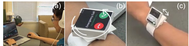
Figure 5. User unavailable: (a) User misses audio notifications when using a headset; (b) Face rotates to indicate an emergency call; (c) Face mimics mouth movement to indicate a lunch appointment.
