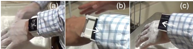
Figure 3. Non-watch hand unavailable: (a) Watch face gets dirty when working in a dirty environment; (b) Face hides inside sleeve to avoid dust; (c) Face moves out of sleeve.
