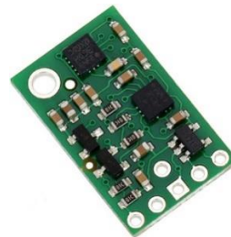
Figure 17: Inertial Measurement Unit
