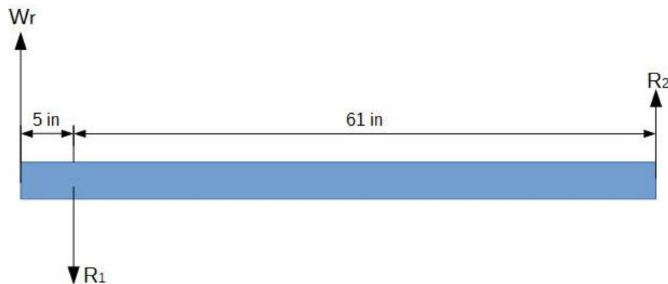
Figure A2: Horizontal loading (y-z axis) on the main shaft.
