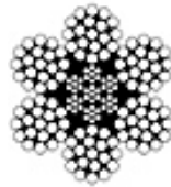
Figure Xx: 6x19 IWRC rope having 15 through and 26 wires per strand
