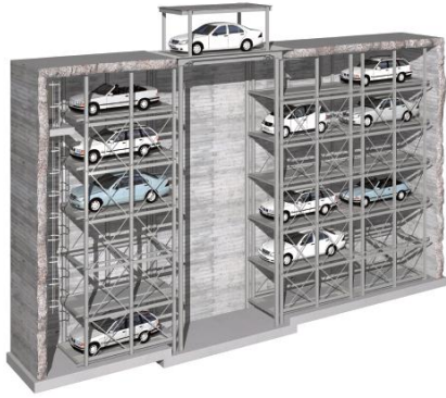
Figure 8 : Cut out view of MasterVario S
