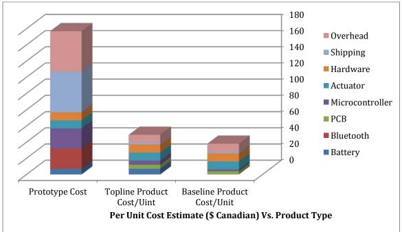
In the above chart the stark price difference between prototype and final products is owing to the development of the prototype using off-the-shelf and third part products. Shipping cost is the single most major fund sink in the prototype, but is predicted to decrease per unit in the final product as a result of bulk shipping. A healthy overhead cost has been included in the prototype so as to contain any setbacks due to component or integration failure.
