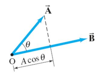
The work done by a force is the dot product between the force and the displacement
