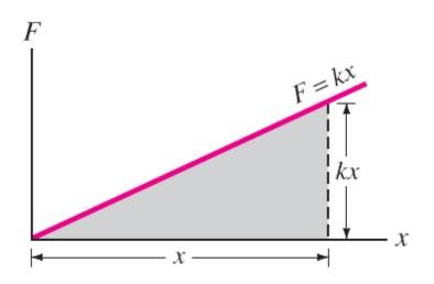
Plot of F vs. x. Work done by the applied force is equal to the shaded area.
