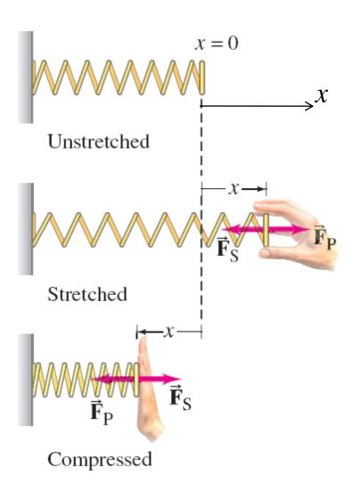
The force exerted by a spring is given by Hooke's law:
