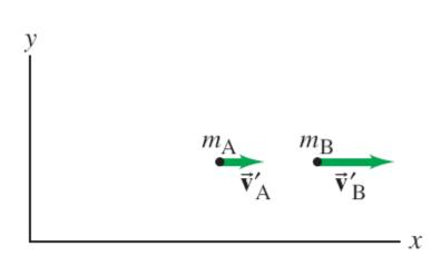
Since both momentum and kinetic energy are conserved, we can write two equations. This allows us to solve for the two unknown final speeds.
