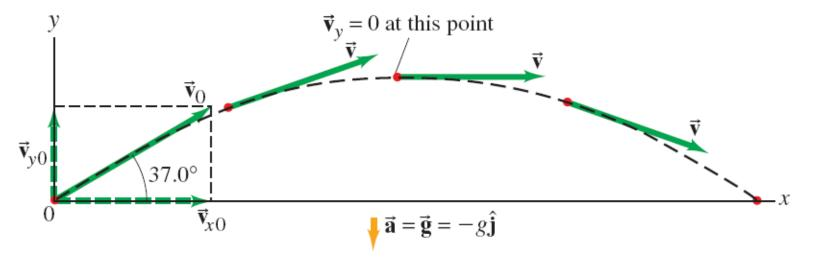
$$v_{x0} = v_0 \cos \theta = 20.0 \cos 37^\circ = 16.0 m / s$$
