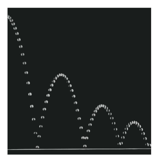
A projectile is an object moving in two dimensions under the influence of Earth's gravity; its path is a parabola.
