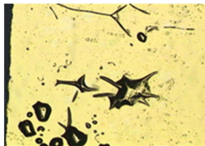
Figure 5.2: Defects in Gold electrode
