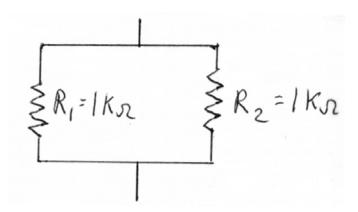
$$\frac{1}{R_{total}} = \sum_{j=1}^{N} \frac{1}{R_j} = \frac{1}{1000} + \frac{1}{1000} = \frac{2}{1000} \dots or \dots R_{total} = 500 \Omega$$
