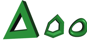
Figure 8: The toroidal polyhedron at three different Catmull-Clark subdivision levels.
