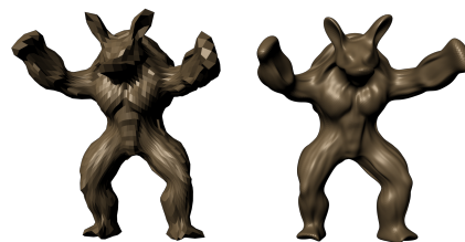
Figure 17: Left: An object obtained from Geometry Images. Right: Left figure after one level of Loop subdivision.
