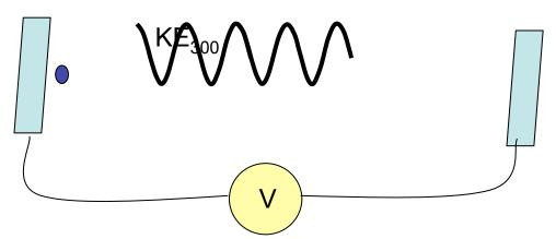
CQ: Shine in light of 300 nm. The most energetic electrons come out with kinetic energy,  $KE_{300}$ . A voltage diff of 1.8 V is required to stop these electrons. What is the work function  $\Phi$  for this plate? (e.g. the minimum amount of energy needed to kick electron out of metal?)
