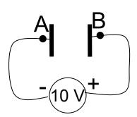
Potential difference between A and B = a. 0 V, b. 10 V, c. infinite volts
