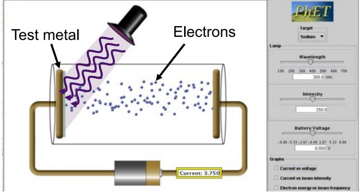
Two metal plates in vacuum, adjustable voltage between them, shine light on one plate. Measure current between plates.
