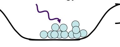
energy needed to kick highest electron out of metal. "WORK FUNCTION" (φ)
