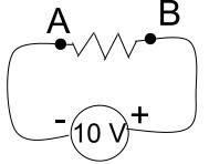
Potential difference between A and B = +10 V Measure of energy an electron gains going from A to B.
