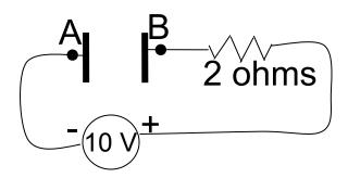
What is current from A to B? a. 0 amps, b. 5 amps, c. 0.2 amps
