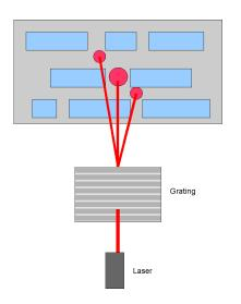
A diffraction grating is used. The central maximum reads the bumps while the 1st-order maxima are used as tracking beams (they should not fluctuate).
