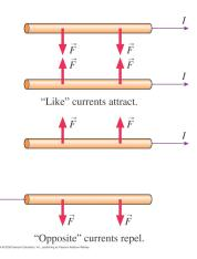
Since we know that current in a wire causes a magnetic field, two wires should act like two magnets...they should attract or repel.
