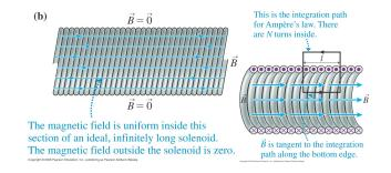
We can use Ampere's Law to calculate the magnetic field inside a solenoid.
