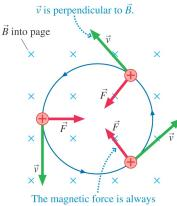
perpendicular to  $\vec{v}$ , causing the particle to move in a circle.
