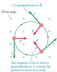
• If you put a moving charged particle in a uniform magnetic field you get the picture at the left.
