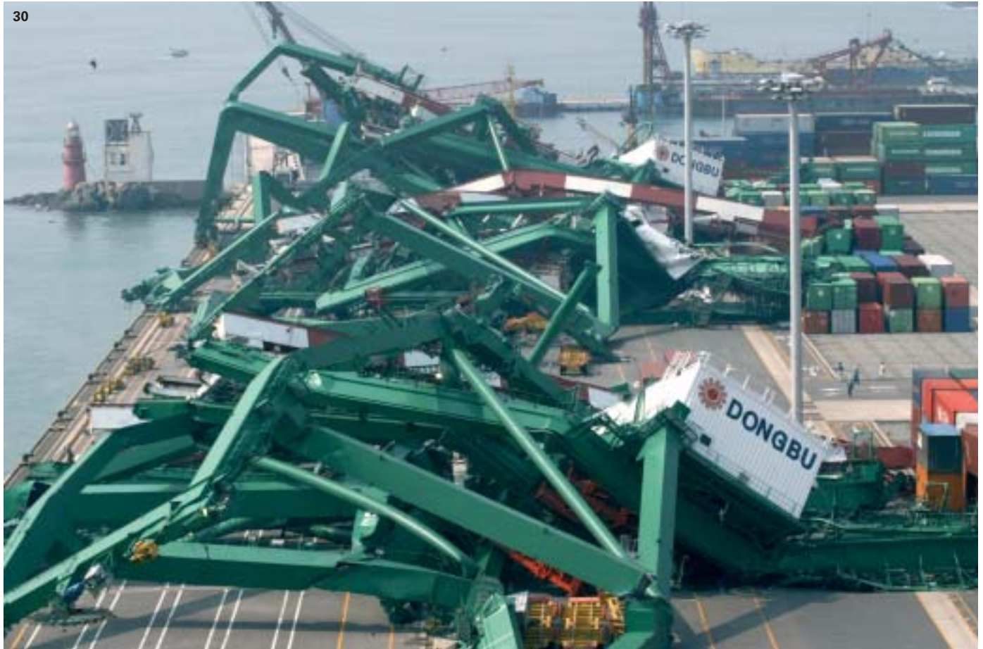
A loading crane toppled by the wind in the port of Pusan.
