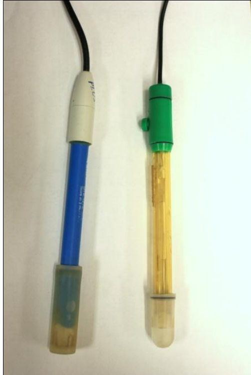
Figure 1: pH electrodes stored in buffer solution held within the electrode storage cap. It is VERY IMPORTANT to store the electrode in pH 4.0 buffer solution when not in use.
