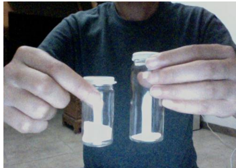
Figure 2: Glass jars: jar on the left represents the ideal amount of sample; jar on the right represents the ideal amount of Borax.
