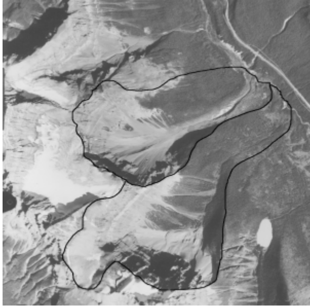
Figure 1-5. A single catchment area or watershed of a drainage basin. Interfluves are delineated with a black line.
