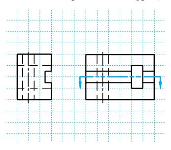
For each exercise listed below, sketch the given views and create a cross-section for the given cutting plane. You should use graph paper for these exercises. Each drawing should occupy half a page.
