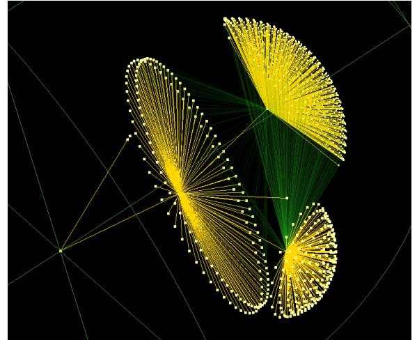
Figure 6. Walrus AS topology graph of the collected BCNET traffic. The centers of the three clusters correspond to BCNET transit providers with AS numbers 852, 6,327, and 13,768. Clusters consist of 683, 588, and 155 AS nodes, respectively.
