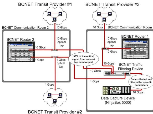
Figure 1. Physical overview of the BCNET packet capture.
