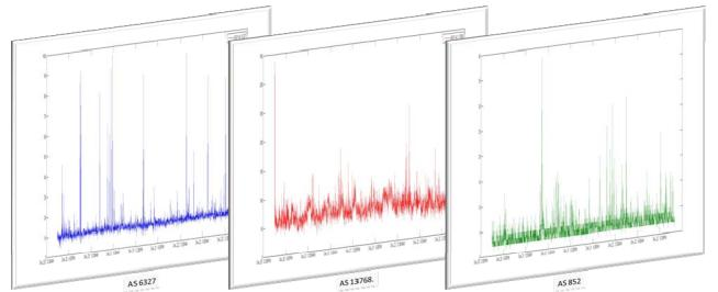
Figure 5. The traffic generated by the BGP update messages for the three BCNET transit providers. Total of 230,424 BGP update messages were identified.
