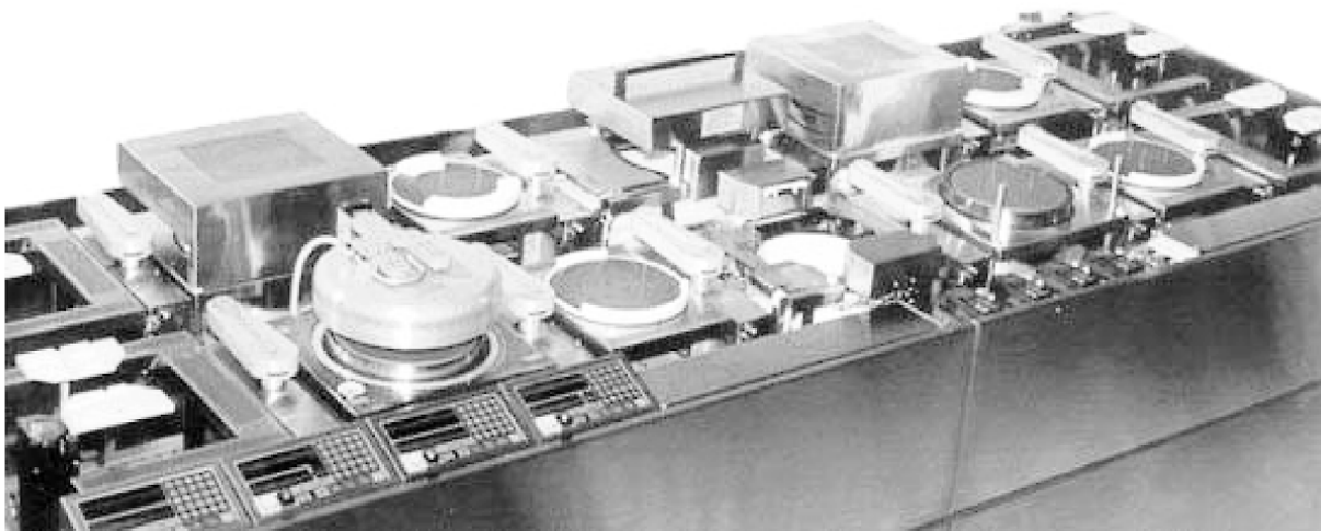
Figure 4-17 A photograph of an automated spin-coater. There are three parallel tracks for processing. At the left-hand end are three "sender" wafer cassettes, partially raised; at the right are three empty "receiver" cassettes that are lowered almost flush with the machine surface. Wafers move from left to right, through the spin and bake modules. A keyboard and CRT screen allow entry and monitoring of process variables. (Photograph courtesy of GCA Corporation, Bedford, Massachusetts. Wafertrac® is a registered trademark of GCA Corporation.)
