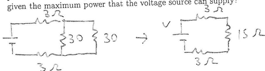
$$P = \frac{V^2}{R_{tot}} = \frac{(10V)^2}{60 \Omega} = 1.67 \text{ W}$$
