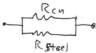
$$\frac{1}{R_{total}} = \frac{1}{R_{Cu}} + \frac{1}{R_{Steel}} = 5.39 \Omega^{-1} \therefore R_{total} = 0.186 \Omega$$
