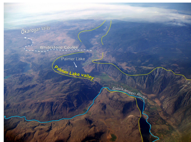
Fig. 13. Southward-looking oblique aerial photograph of Similkameen Valley and Palmer Lake Valley. The modern course of the Similkameen River makes a sharp east-northeast turn in a wetland area north of Palmer Lake. Palmer Lake valley is a bedrock valley with modern underfit and ephemeral streams. It may have operated as a tunnel valley during glaciation. Smaller bedrock coulees like Whitestone Coulee branch off toward Okanogan valley.
