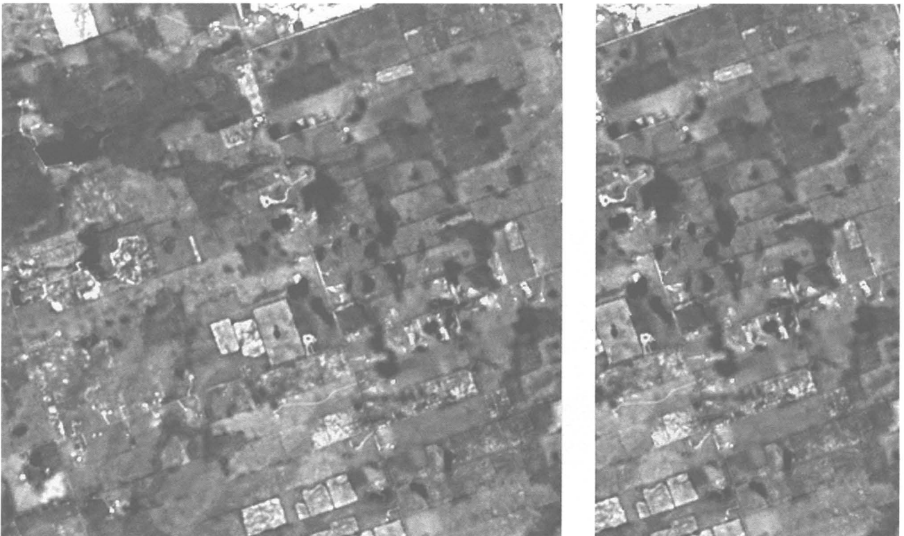
Figure 5. Stereo-Pair showing hummocky terrain on the south central flank of the Oak Ridges Moraine. Imagery generated from merged Landsat TM, a SPOT Panchromatic image and a DEM.
