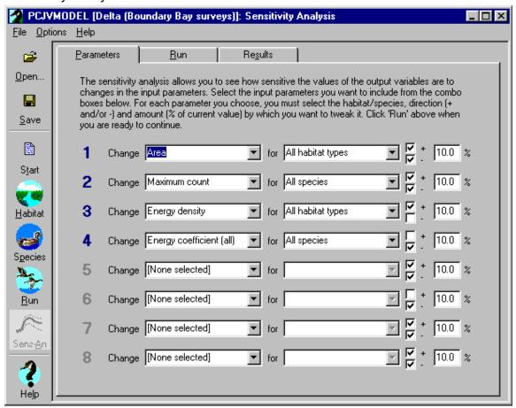
The sensitivity analysis provides the user with a way to explore the sensitivity of the output variables to deviations in specific input parameters. Deviations in input parameters may reflect actual variability in those parameters, or uncertainty in their true values.
