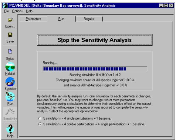
On the *Run* screen under *Sensitivity Analysis*, you must first specify whether to change each parameter individually (single perturbations), or to include all possible pairings of parameter changes (double perturbations) as well. Press the *Run Sensitivity Analysis* button to start the sensitivity analysis. You can press the button, *Stop the Sensitivity Analysis*, to abort it. Once it is finished, press the *Results* tab (see below) to see the results.
